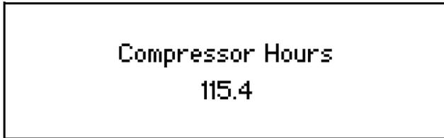
3. The cumulative hours of concentrator operation (compressor hours) will be shown on the display screen for as long as the button is continually pressed. The concentrator run time is displayed to the nearest 0.1 hours.
