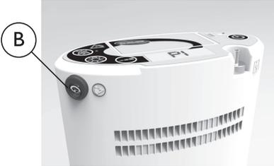
A side view of the oxygen concentrator. A circular AC power input connector, labeled 'B', is located on the left side of the device. The device is white with a control panel on top and a vented front.                                                                  |
