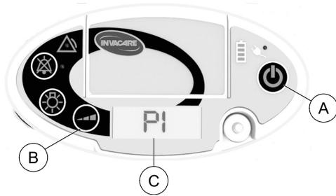
1. With the concentrator running, press the flow selection button **B** to increase the pulse flow setting by one increment.
