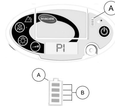
The battery gauge ① shows the status of the installed battery charge level when the concentrator is turned on and when the concentrator is off but connected to an external power source. The number of illuminated segments ② of the battery gauge ① indicates the charge level of the installed battery. If two batteries are installed the indicated charge level is that of the least charged battery.
