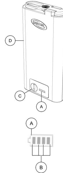
When the battery ④ is removed from the concentrator, press the battery status button ③ to show the status of the charge level on the battery gauge ①. Refer to the charge level ② table in Reading the Battery Gauge for Installed and Uninstalled Battery(s) in Setup.
