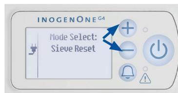
13. Press the alert
