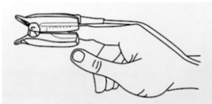
Figure 5-1 Placing the Adult SpO<sub>2</sub> Sensor
