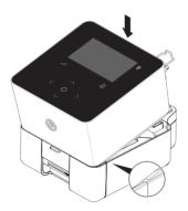
5. Connect the power mains cable to the device. Secure the power cable to the device with the help of the safety clip. Insert the other end of the
