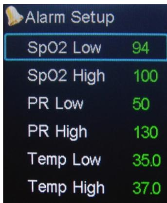
Figure 4.4.3 Alarm setup menu
