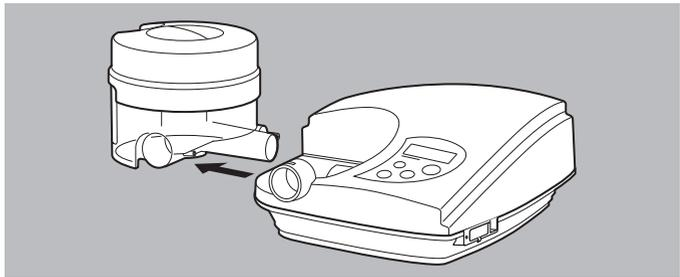
1. Push the humidifier sideways out of its locator.
