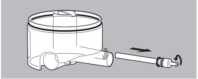
2. Unscrew the heater rod from the lower part of the housing.
