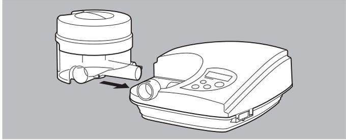
4. Push the humidifier into the locator for it on the side.
