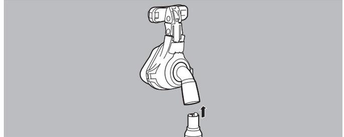
4. If not integrated: connect the external exhalation system between the breathing mask and the breathing tube.
