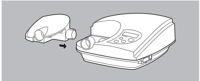
2. Push the cap into the locator for the humidifier up to the stop.
