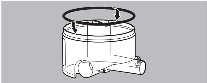
3. Push a new seal into the groove for the lower part of the housing.
