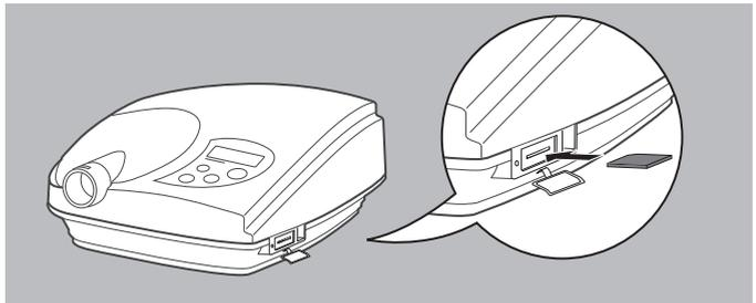
2. Push SD card into SD card slot until it engages. In the process, please note: the missing corner of the SD card must face front right when you push in the card.
