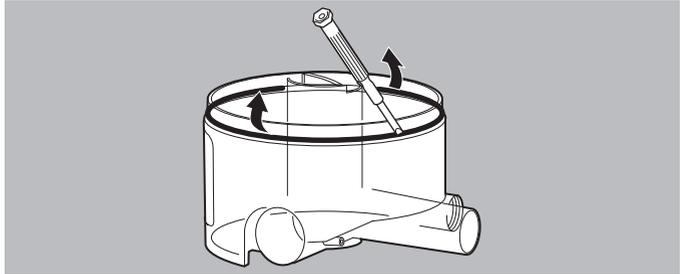
2. Use a screwdriver to remove the seal carefully without damaging the groove.
