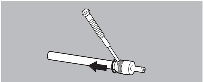
3. Use a screwdriver to remove the seal carefully without damaging the groove.
