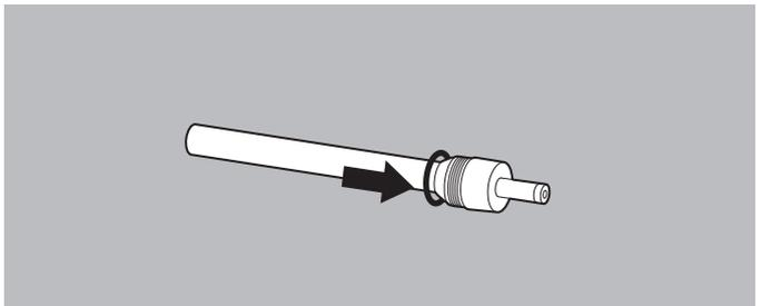
4. Push a new seal into the groove for the heater rod.
