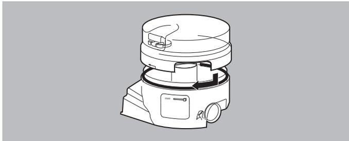
7. Screw together the parts of the housing.
