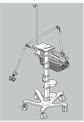
You can use the oxygen cylinder clamp with oxygen cylinders up to 120 mm in diameter (this corresponds to a cylinder size of approx. 4 l to 6 l per cylinder). Note total cylinder height (cylinder including valve and accessories).
