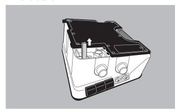
3. Remove filter for cooling air fan.
